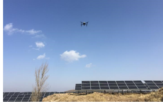
Figure 1. The illustration of PV inspection using an UAV
