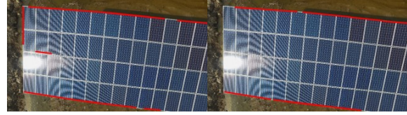
Figure 8. Boundary lines through Hough transform and screened ones
